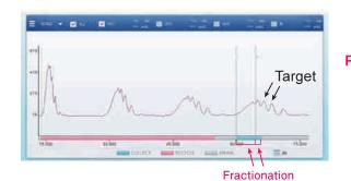
Preview Function enables to find and avoid error setting for fraction collection easily.
