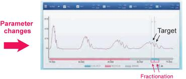
After the change of method parameters, you can check if the new fractionation window works.
